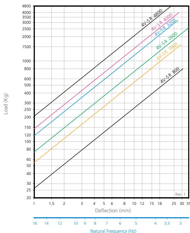
LOAD VS DEFLECTION DIAGRAM AMC-MECANOCAUCHO® 4V-SR
