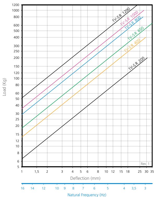
LOAD VS DEFLECTION DIAGRAM AMC-MECANOCAUCHO® 1V-SR
