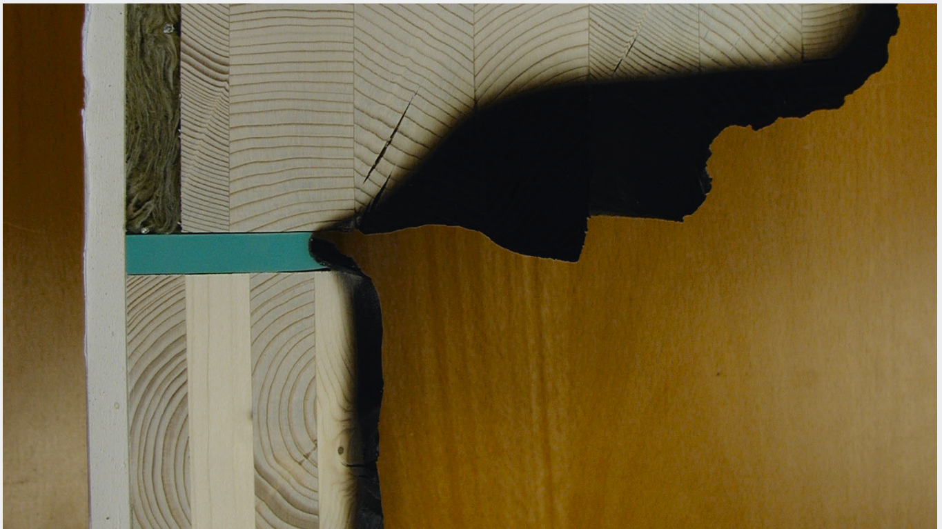
Fig. 7: Connection detail after exposure to fire for 60 minutes
